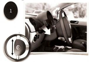
To begin, release the wheel locking mechanism and pull it down and out. Then turn the wheel so that the two sliver spokes are vertical.
