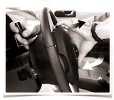
Slight pressure on unlatched side of the airbag may be required to fully release the air bag in step 6 when working on second hold. Once spring is disengaged, remove airbag.
