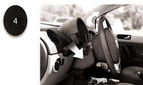
Insert removal tool with the tip as close to the rim side of the hole as possible. Then engage tool tip behind spring.
