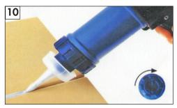
**10. Applying beading without spraying** The spray air is to be turned off if a bead of material needs to be applied.
