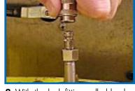
**2.** With the lock fitting pulled back, slip over the connector on the fluid container.
