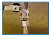
**4.** Complete the connection and let the lock fitting go. It will automatically slide into place and make the fitting secure. (If the whistling continues, the connector may need to be replaced).
