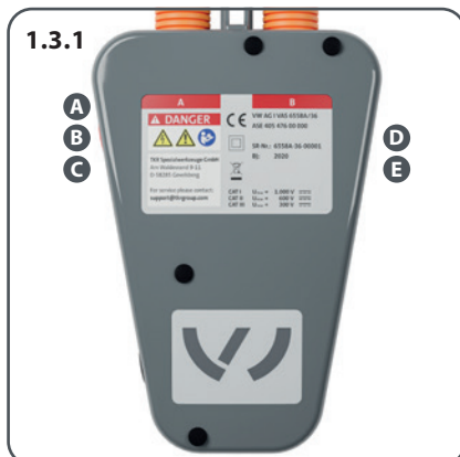
1.3.1 Markings on top of the high-voltage test adapter
