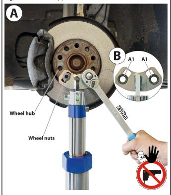
Fig. 4: Lock the camber angle adjustment.
