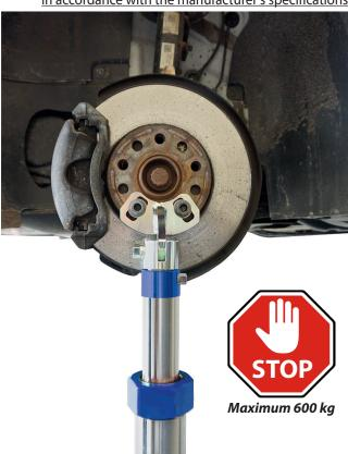
**Fig. 6:** Relieve the support device and remove it from the wheel hub.
