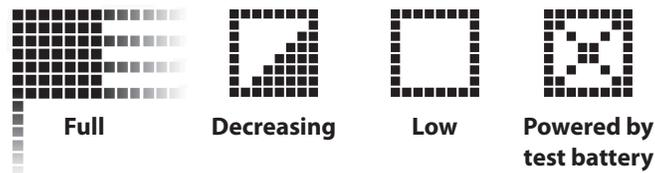
Figure 7: Power Level Indicator for AA Batteries
