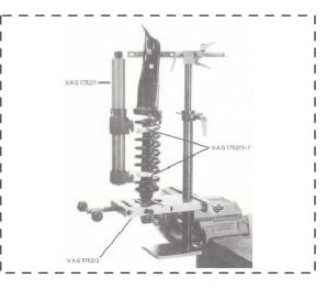
This universal device can be used to service all suspension struts from Volkswagen and Audi passenger cars.
